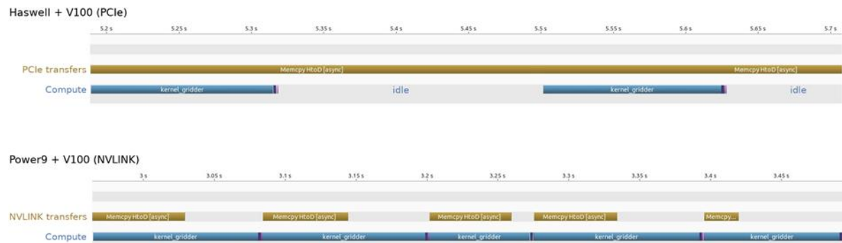
Figure 5: Timeline of the imager application. PCIe transfer rates of 12.5 GB/s are not sufficient to keep the GPU busy (top figure), while NVLINK transfer rates of 68 GB/s are (bottom figure).
