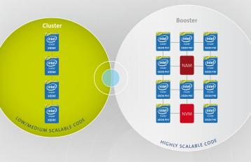
The highly scalable code parts of an application run on the Booster, while those code parts with limited scalability benefit from the large single-thread performance of the Cluster. This code division ensures an optimal use of the system.
